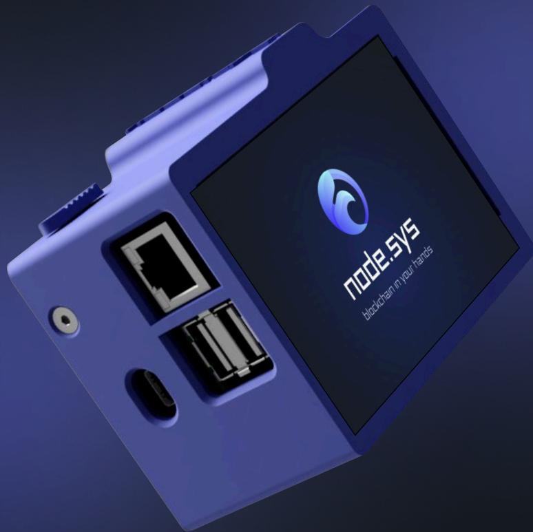
The core element **Node.sys** is a backbone hardware node. This is a ready-made hardware solution based on publicly available components, which can be self-assembled and the device case printed on a 3D printer. The hardware node processes transactions on a decentralized network and generates blocks, thus supporting the blockchain network.
